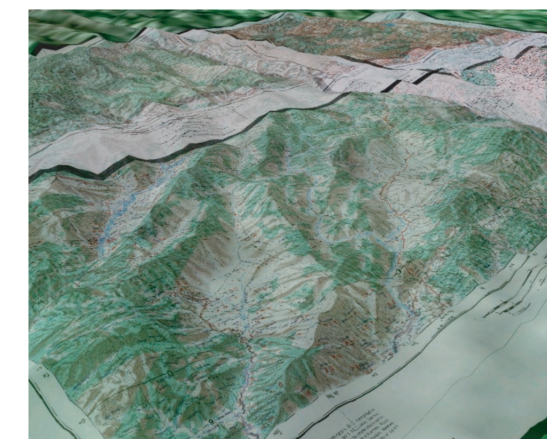
Army Map Service 1:500 Series of China topographic maps, georeferenced and draped over GTOPO30 elevation data. The 3D effect was done with ESRI ArcGlobe software, with the terrain model exaggerated by a factor of 2.
