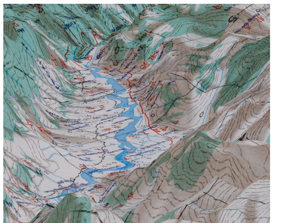
Army Map Service 1:500 Series of China topographic maps, georeferenced and draped over GTOPO30 elevation data. The 3D effect was done with ESRI ArcGlobe software, with the terrain model exaggerated by a factor of 2.
